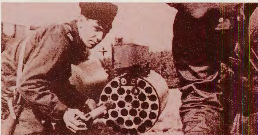
Ground crew loading helicopter's main battery — 57mm S-5 HE rockets — into 32-tube rocket pods. Photo: Courtesy David Isby
